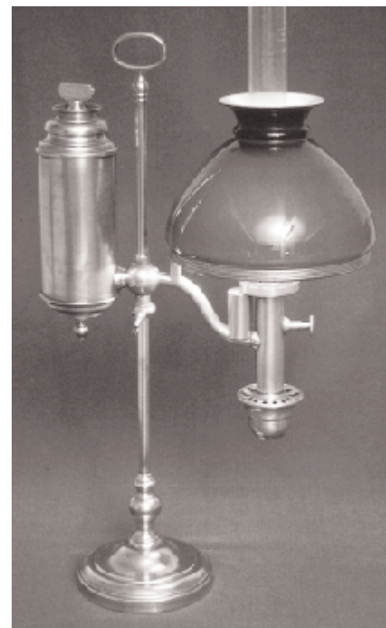
Figure 5.1 An early oil lamp that used colza oil, a design that has been much copied and converted to electricity. (Copyright Science Museum, London)
